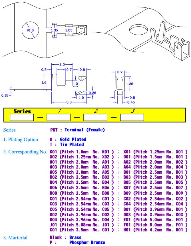
EXAMPLE : PXT T B01 Terminal (Female) For Pitch 2. 5mm Tin Plated (Serial number : B01)
